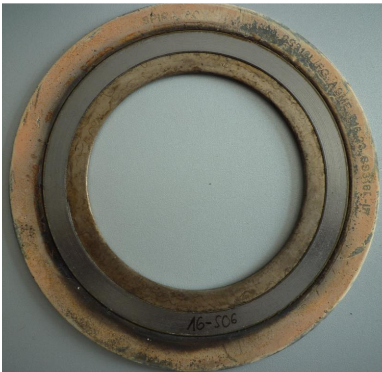
Fire test according to API 6FB (MESC SPE 85/300 - 3.3.3)
