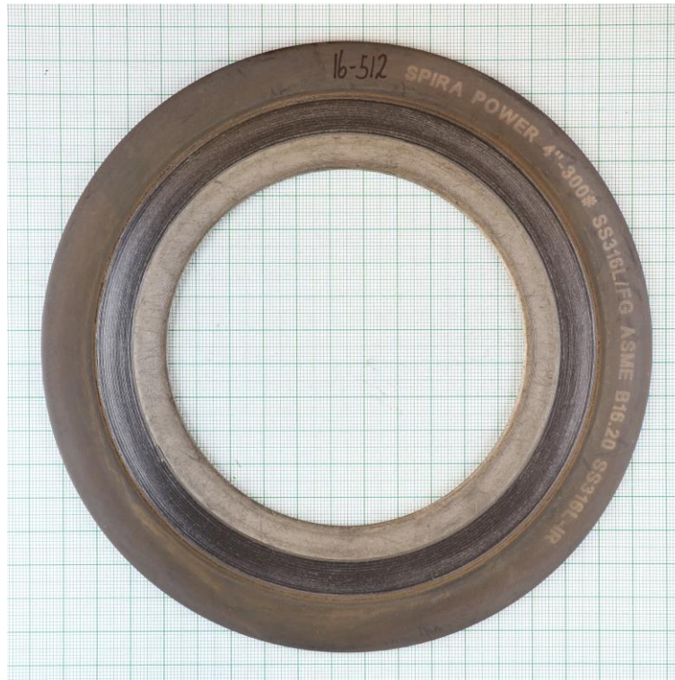
Shell cycle test (T) according MESC SPE 85/300 - 3.3.5
