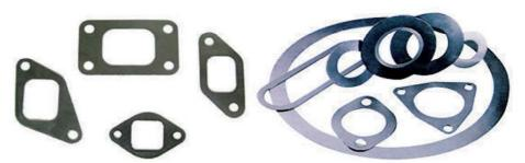
Graphite gaskets are used in processes that include corrosive media like ammonia, hot water, high pressure vapours, ultra cool liquids and hydrocarbons. This can withstand a temperature -200°C to 650°C This makes them the top choice for heat exchangers, cooling towers and high pressure pipes. Spira Power provides gaskets fully customized to your dimensional and mechanical requirements.
